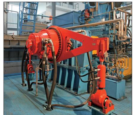
This rubber mixer is driven by Häggglunds new flexible and modular drive system Gemini. The drive motor range CBP can provide power from a single unit of over 1000kW with speeds over 300 rpm and torque up to 250kNm.
