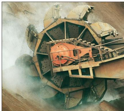
Bulk handling applications like bucketwheels, feeders and conveyors need a drive which is reliable in all environments. With full torque from zero to max speed and low inertia gives fast response and protects equipment from overloads.
