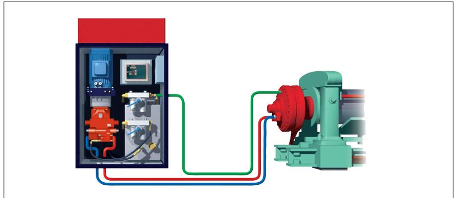
A typical Häggglunds Drive consists of a drive motor selected from the wide range available to give the torque required. A power unit with a variable displacement pump/motor set and necessary tank, filters and instrumentation. A control and monitoring unit and the inter piping. The arrangement is versatile and flexible which enables customisation to suit the exact requirements of the application and environment.
