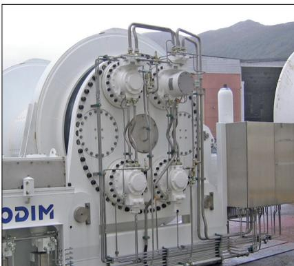
The Compact motor is ideal for high powered winches where several motors can be utilized as required in a modular design. We have brakes, valves and other accessories to ease applying to marine applications.
