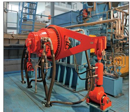
This rubber mixer is driven by Hägglunds new flexible and modular drive system Gemini. The drive motor range CBP can provide power from a single unit of over 1000kW with speeds over 300 rpm and torque up to 250kNm.
