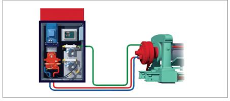
A typical Hägglunds Drive consists of a drive motor selected from the wide range available to give the torque required. A power unit with a variable displacement pump/motor set and necess-sary tank, filters and instrumentation. A control and monitoring unit and the inter piping. The arrangement is versatile and flexible which enables customisation to suit the exact requirements of the application and environment.
