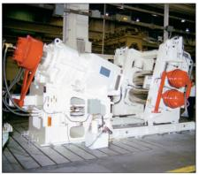
Rubber processing machines like this extruder-sheeter or mills and internal mixers improve productivity with direct hydraulic drives. They are responsive, forward/reverse and fast stop, giving full torque even at the very low end of speed range with through hole facilities for cooling water.
