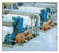
Process applications like displacement or screw presses are ideal for direct hydraulic drives. The speed can be controlled in relation to load to improve the performance. The power unit can be positioned conveniently away from the machine improving operator and maintenance access.
