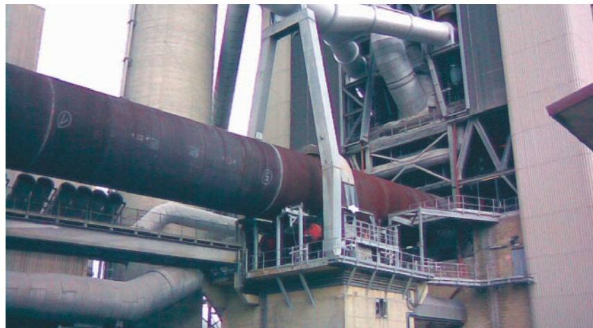
The kiln, manufactured by Krupp Polisiaus is 62 meters long and 4.64 meters in diameter.
