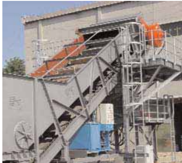
Hägglunds Maraton motor driving a Scraper Chain Conveyor. Many of the Ash Conveyors delivered with Hägglunds drive systems are used in India, China and Malaysia.
