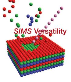
**SIMS** is a high sensitivity surface analysis technique for the determination of surface composition, contaminant analysis and for depth profiling in a sample's uppermost surface layers.
