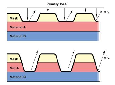
The intensity of the most significant peaks from the mass spectra are plotted against time in Trend analysis giving real time etch depth information
