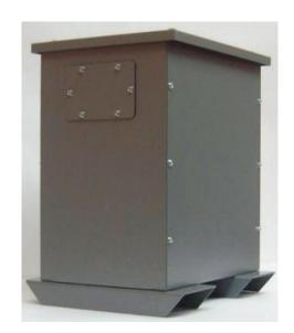
Enclosure to IP44 Made form zinc plated sheet steel Powder coated with polyester paint Gland plates are removable Gland plates must be detached from box if drilling of cutting gland holes Enclosure base has skids for forklifts Ventilated for transformer cooloing
