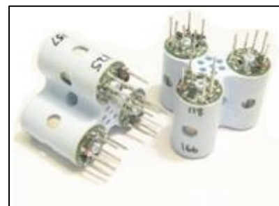
Low Profile Array technology integrated into a 25mm Ø triplet configuration
