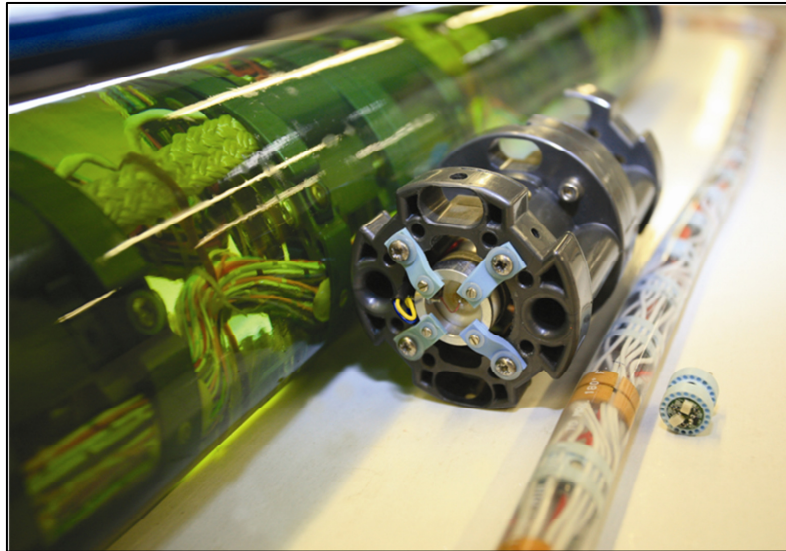
Comparative size of a n 89mm Ø conventional Line Array and the 16mm Ø Low Profile Array
