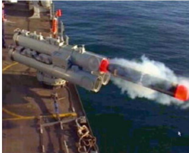
Deck mounted variant showing launch of Sting Ray torpedo
