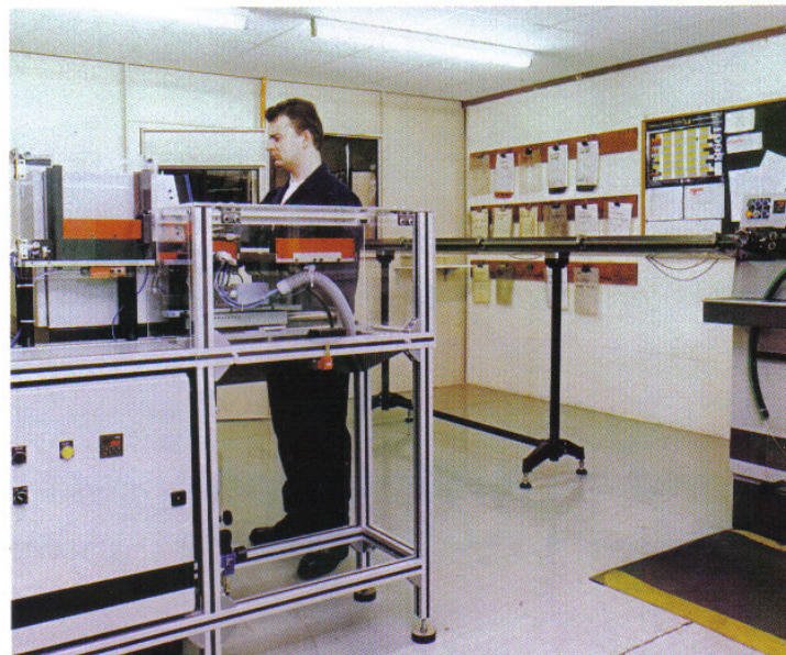
Fine wire straightening machine and automatic cassette collection.
