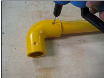
Pop rivet fittings into place with M4 x 20
