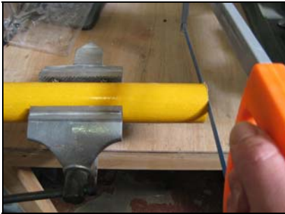
Cut tubes to length with hacksaw
