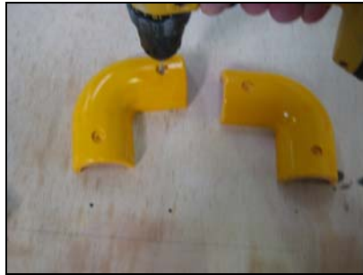
Drill out rivet holes on fittings with 4mm drill
