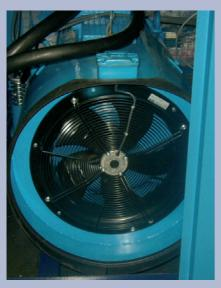
AC drive motor, TEFC IP55, 4-pole, with separate fan ensures full cooling at all operating conditions. Low thermal motor load, insulation class F, insulated bearings
