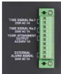
External alarm terminal
