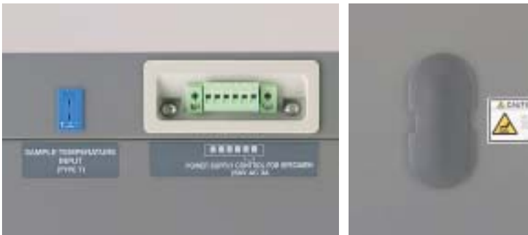
Specimen temperature input (Left) Specimen power supply control output (Right)
