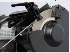
Produces a longitudinally ground taper with a 20RMS finish and a +/- 1/2° angle tolerance.
