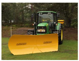
MK1 PA, Straight Vee 3000mm Blade Width In Straight Position.
