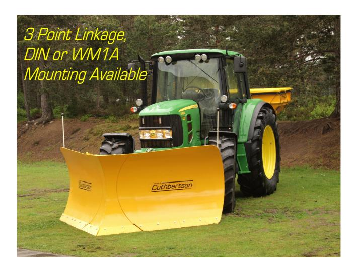
4 Position Operation Controlled From The Cab.
