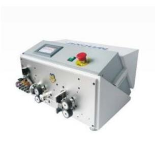
Automatic measurement of wire diameter. Automatic opening and closing rollers. Wire Size - AWG 10 - 30 Stripping Length - 0.1 - 40mm Capacity (L=100mm) - 103pcs/min
