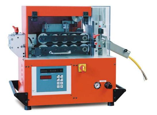
The Autocut 20 / 85 B QC and 30 / 85 B QC is an electro-pneumatic Cutter for materials to max. 25 and 30 mm in diameter or Max. 85 mm width (depending on material). A quick-change facility allows a simple retooling to different requirements, such as cutting of cables, stranded wire, tubing, corrugated, wire ropes, Bowden cables, plastic pipes, thermal cutting or grinding separation. Standard Volume distance limitation.
