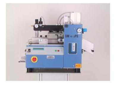
The SM15 2PS has a powerful stepper motor. The cutting length accuracy is approx. 1/10 of a millimetre. The machine can be used for a wide range of materials, such as: PVC hoses, fabric hoses, flat cable, round cable, wire, stranded wire, foil, soft rubber, hard rubber, PVC profiles, wire mesh, textiles, paper etc.
