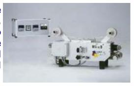
The Material feeding is by a SM15 or a cut and stripping machine. The print impulse is an potential free contact. The temperature and printing time is regulated in a separate electronic box.
