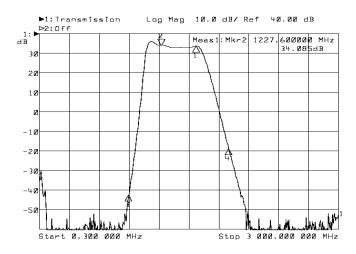
The above picture shows the GPS-BNC frequency response from 300 kHz to 3 GHz. Ultimate rejection is typically > 80 dB
