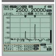
The Dalta Marker is displayed on the same position as that of the normal marker, The frequency and level value of this marker are relative to those of the nomal marker.
