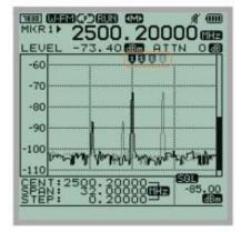
This function sets the marker at peak within the search range, and the marker frequency (at the peak point) is then set to center frequency.
