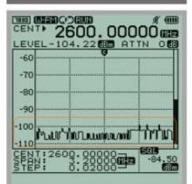
7830 supports -110dBm of low displayed average noise level. Noise is extremely important for measurements on frequency-processing equipment or when searching for Interference signals.
