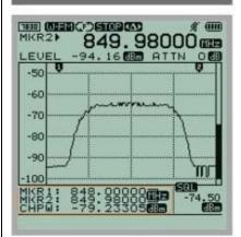
The Channel power Measurement Function is for determining the power in a transmission channel specified by the user, In the case of CDMA with 849,98MHz channel width at 1,25MHz from the carrier,
