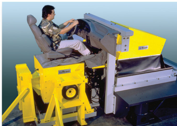
Ford's VVS dual CUBE system for simulating the vibration response of a vehicle to recorded road data. Used for the subjective evaluation of ride quality.
