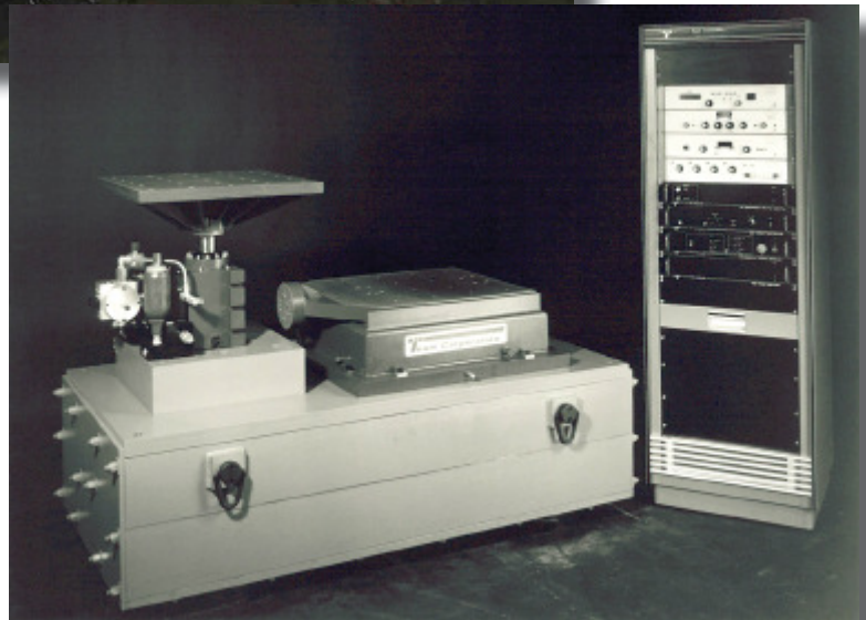
Figure 4. These archival photos illustrate a common system configuration. The actuator is designed to mount both vertically for use with a Specimen Mounting Plate (SMP) and horizontally for use with Team's patented T-Film slip table system. The actuator and slip table are mounted on a common reaction base which can be configured to meet customer needs - movable, airbag isolated or fixed.
