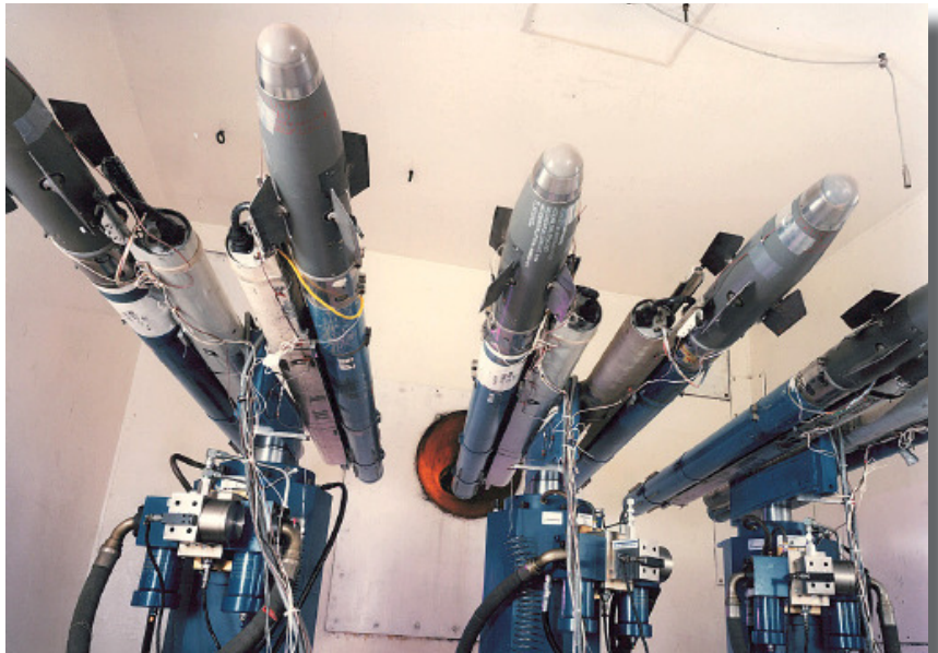
Figure 3. Multiple Team vertical actuators mounted in an acoustic reverberant chamber used to duplicate the acoustic and acceleration loading of under wing mounted munitions systems.
