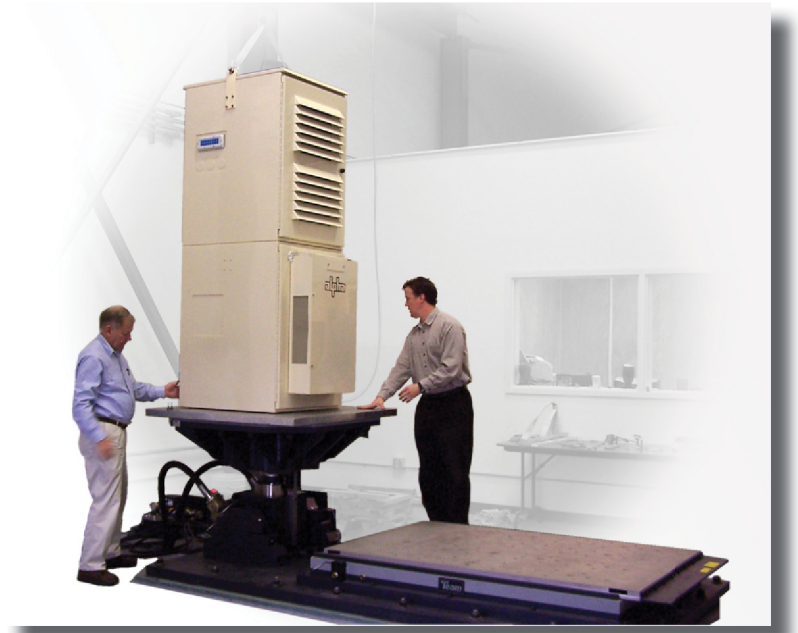
An example of a large cabinet being installed on Team's SSTS, prior to testing in the vertical direction.
