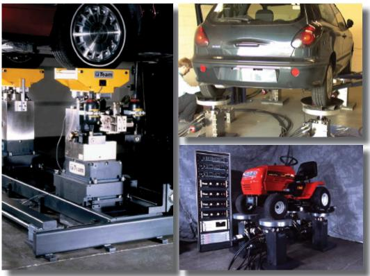
Team Four Poster Systems are designed as fixed-in-place or portable depending upon your requirements. Actuators are available with standard P-P displacement of two (2) or four (4) inches. Longer displacement actuators are available to fit custom applications.
