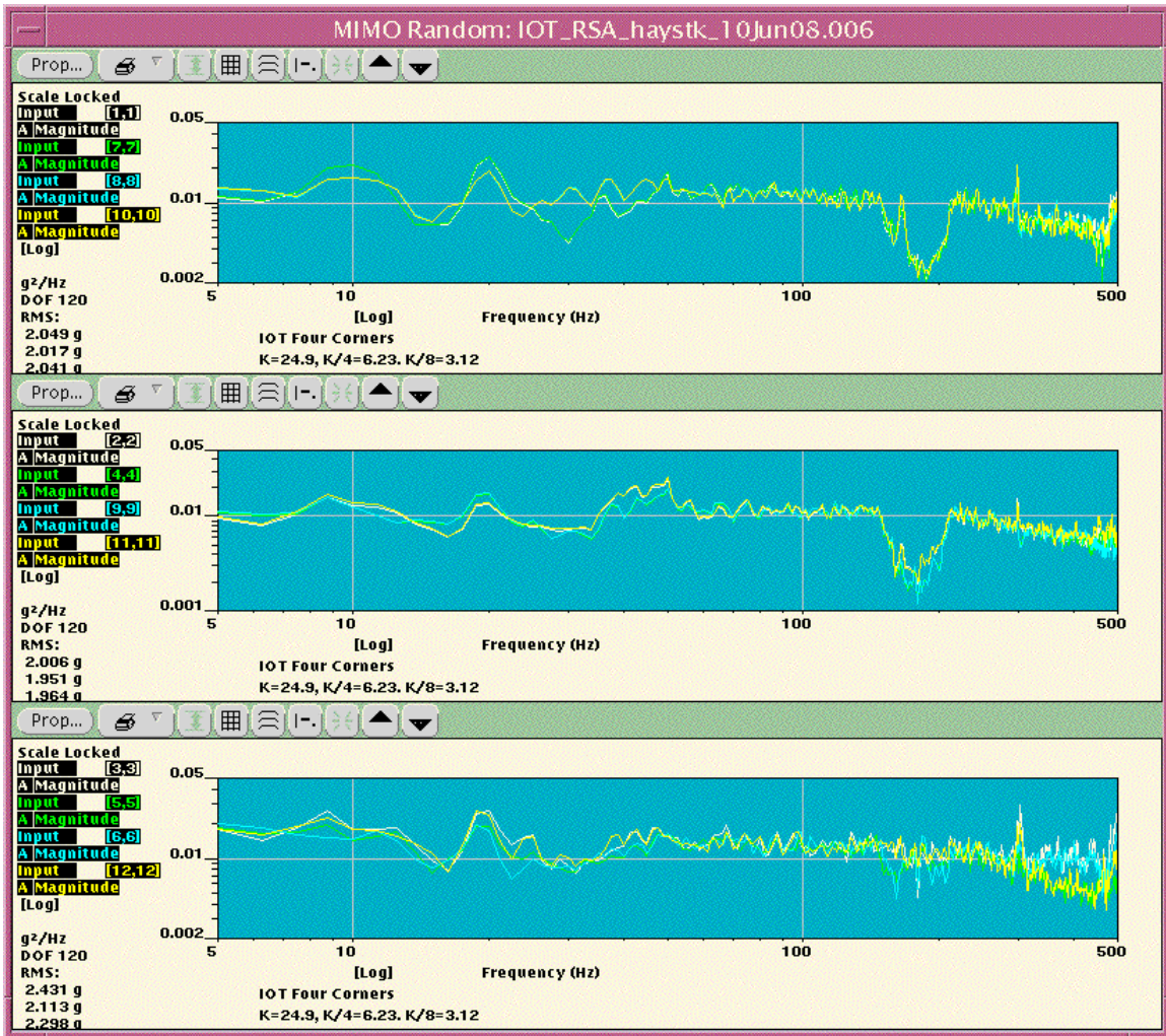
Fig. 19: PSD Responses for the Control Inputs for Test 8
