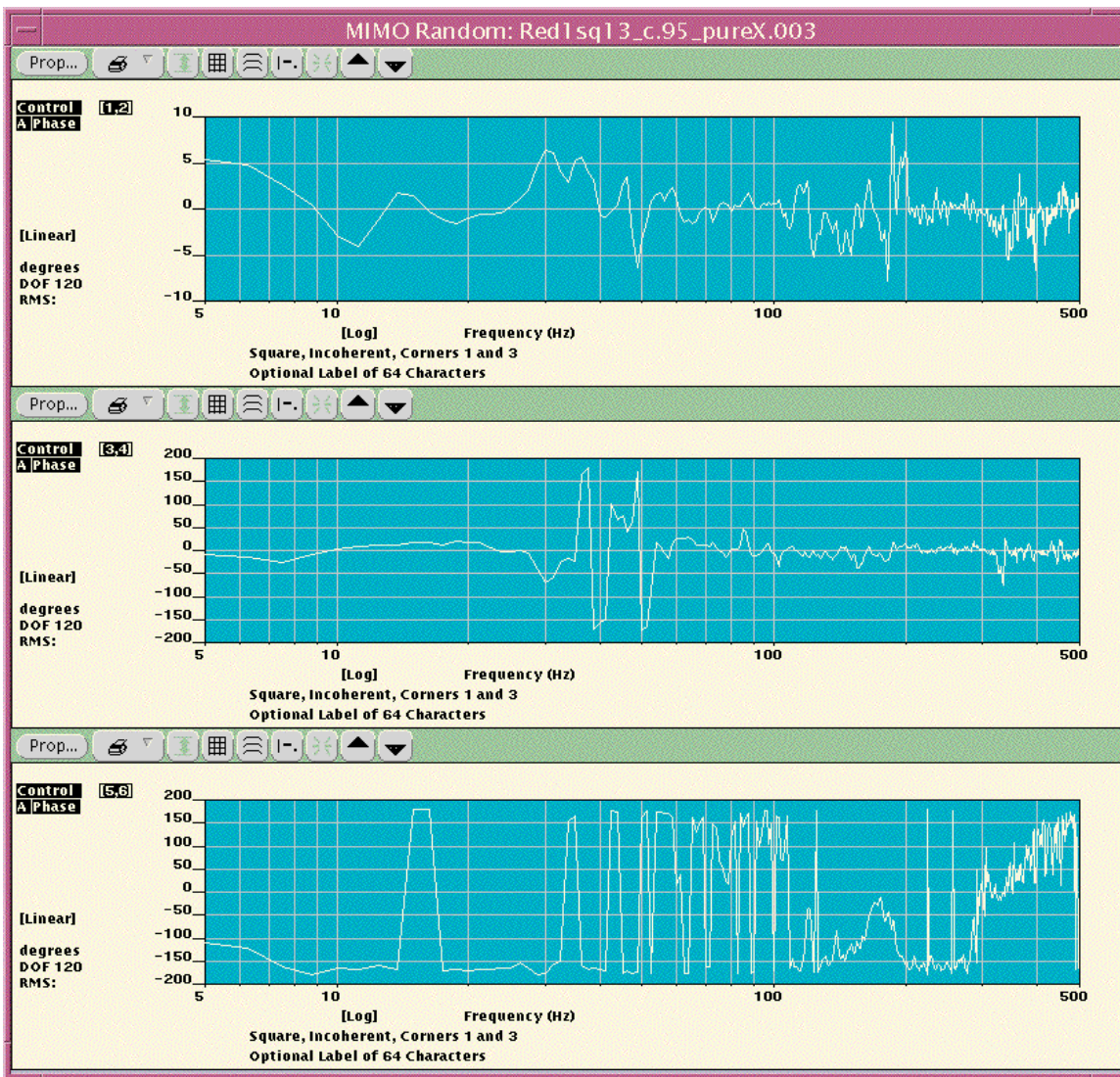
Fig. 9: Phase Response Between Like Axis Control Accelerometers for Test 3
