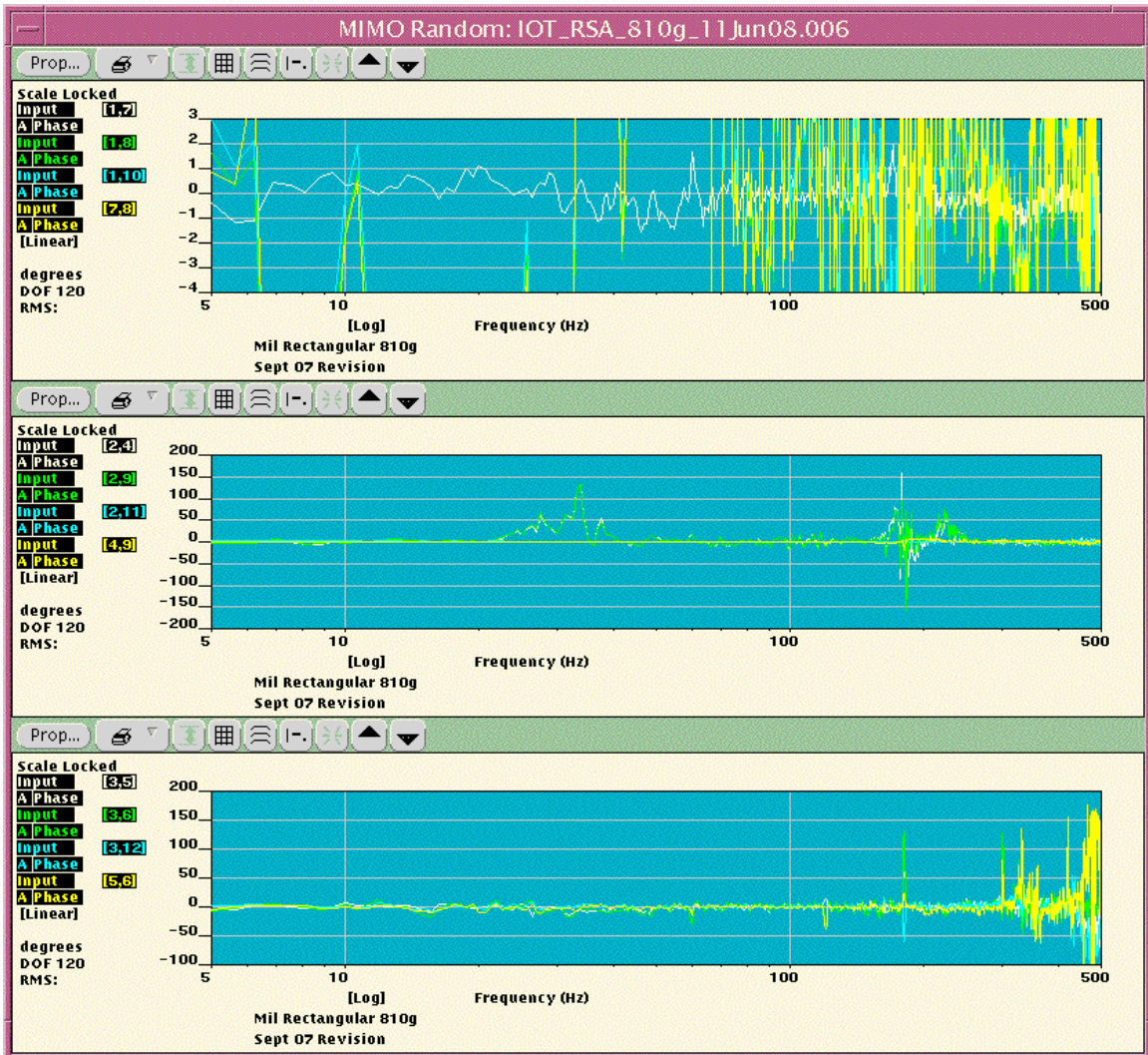
Fig. 25: Selected Phase Responses Between Control Inputs for Test 9
