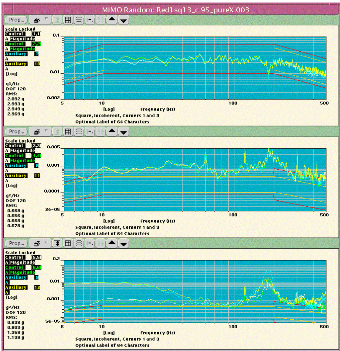
Fig 8: PSD Responses for Auxiliary and Control Accelerometers for Test 3
