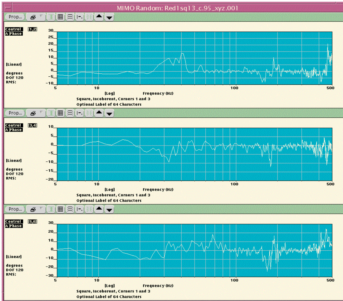
Fig 7: Phase Response Between Like Axis Control Accelerometers for Test 2
