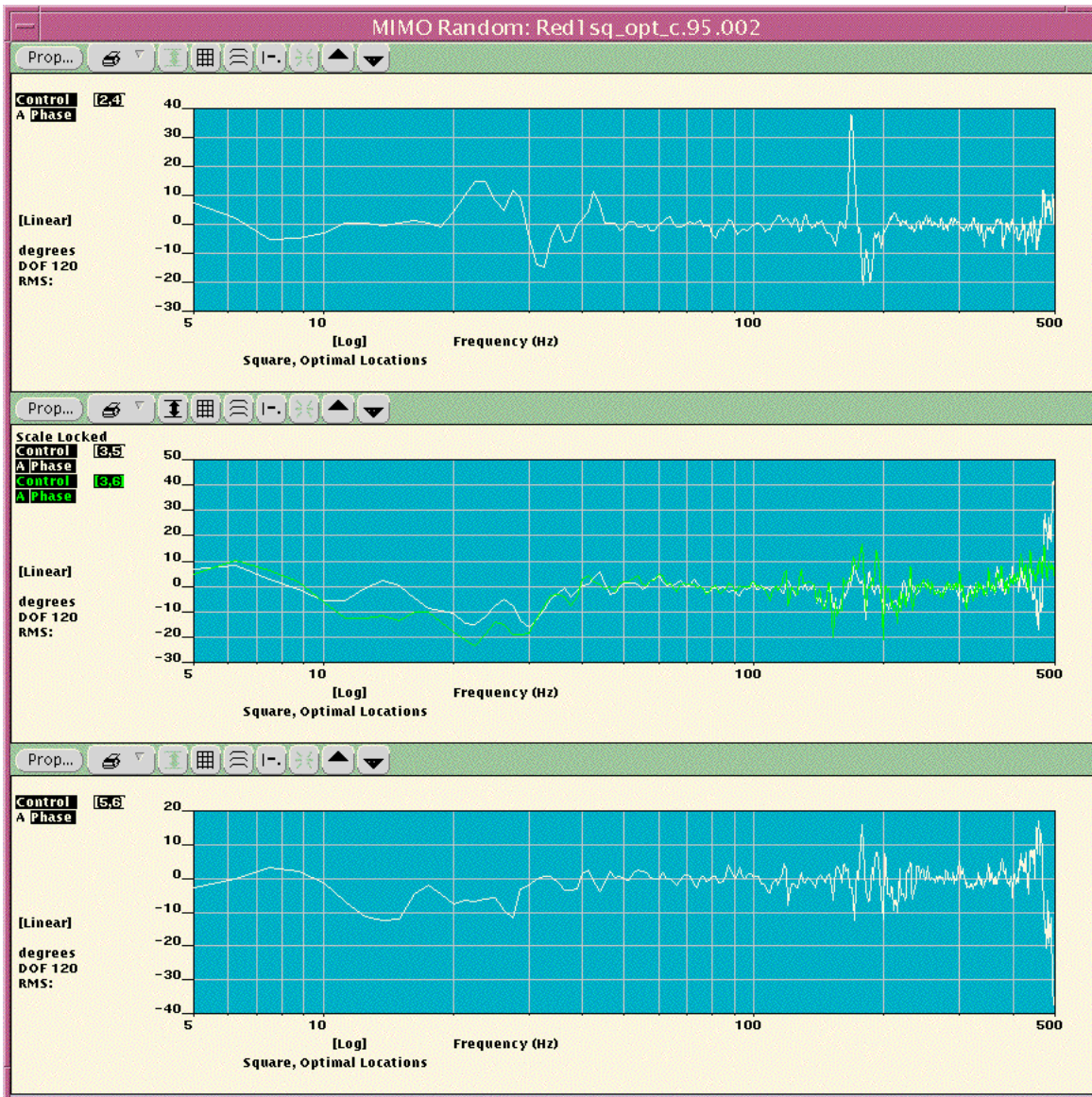
Fig. 12: Phase Response Between Like Axis Control Accelerometers for Test 4
