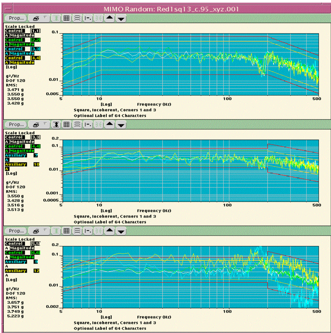
Fig 5: PSD Responses for Auxiliary and Control Accelerometers for Test 2
