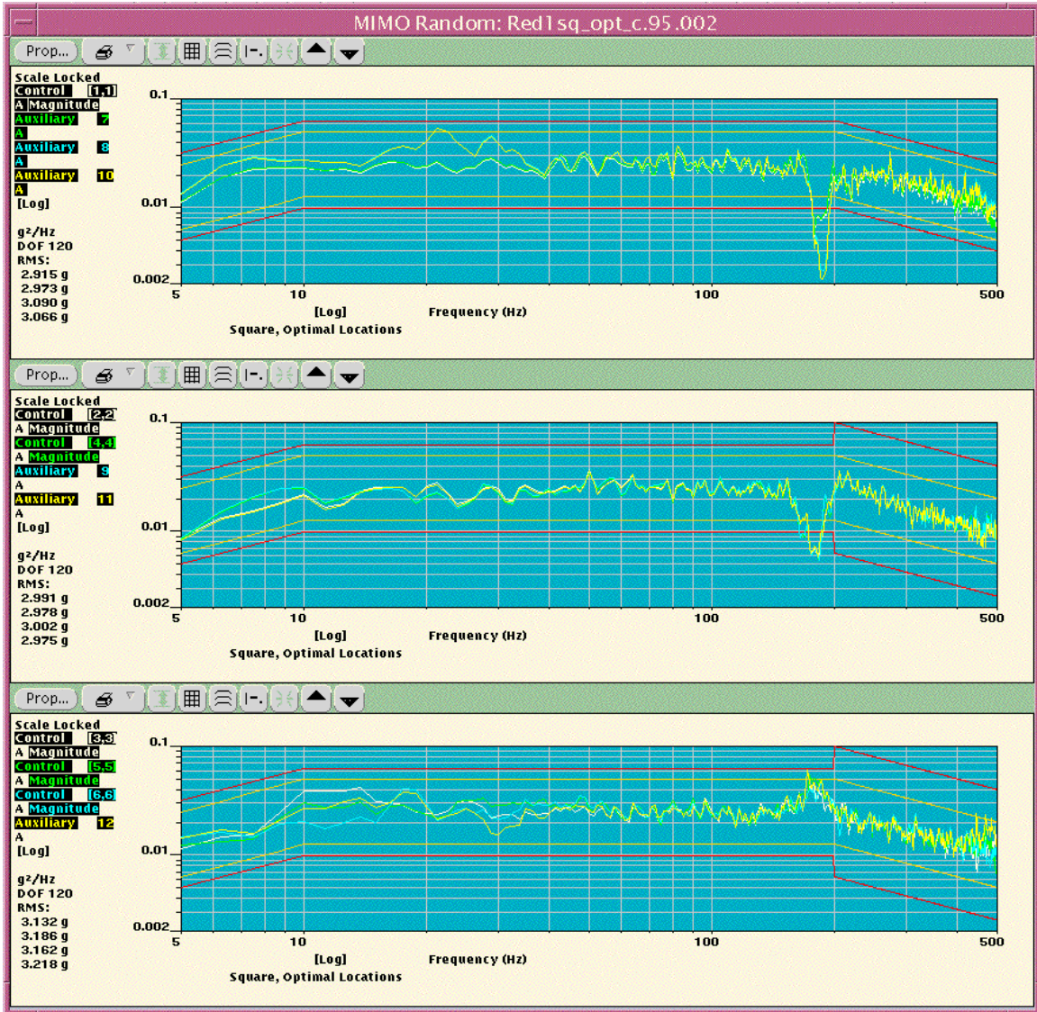
Fig. 10: PSD Responses for Auxiliary and Control Accelerometers for Test 4
