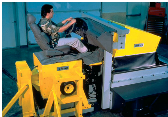
Figure 2: Vehicle Vibration Simulator used for subjective evaluation of ride quality. Photo courtesy of the Ford Motor Company.
