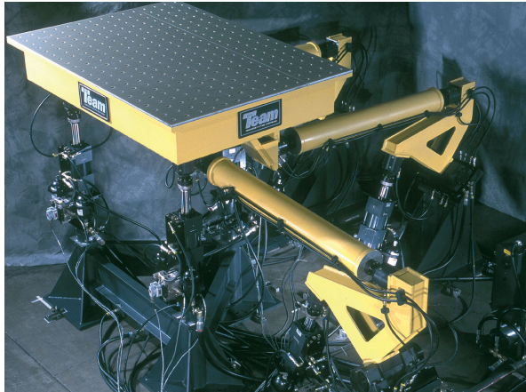
Figure 4: The Mantis™ multi-axis shake table. Hydrostatic bearings are located at the ends of actuators, connecting rods and at the bell crank base mounts.
