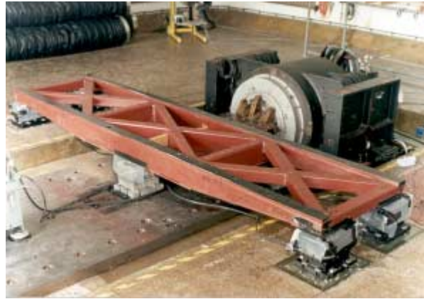
Figure 1.0 Typical single axis vibration test system with ED shaker and linear hydrostatic bearings
