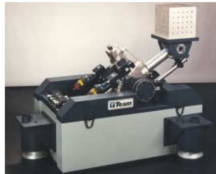
Figure 2.0 Simultaneous bi-axial vibration system used for qualifying small electrical components to IEEE-344.
