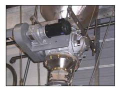
The installation included strengthening the hopper support members, fabricating a more durable mounting flange for the airlock and several transitions to mate to the metal detection unit directly below the airlock. With the installation of the rotary airlock, the capacity has more that doubled and will be able to meet additional needs for many years in the future.
