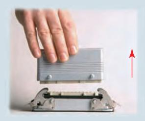
Remove the mobile connector from the fixed connector.
