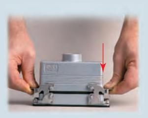
Lower the levers until the locking mechanism is released.
