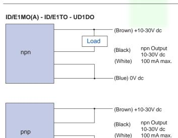
With 4 wire units **connected as shown** above, **output** will be **ON** when unit is **sensing**. For **output OFF** when **sensing**, **reverse supply** wires (only).
