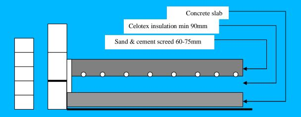
Recommended insulation would be a minimum of 90mm foil faced board with thermal conductivity below 0.019 W/m such as Celotex®.
