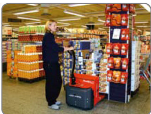
Panther Mini (capacity 1400kgs) is recommended for easy pallet transport, eg in supermarkets and stock areas
