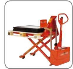
Level control (optional extra) ensures a constant working height.
