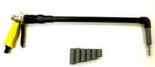
The total length of the filling pistol is 625 mm and it is supplied with a kit of eight spacer tubes so that the probe depth can be accurately set to suit the ranges of Alcad And Saft cells.
