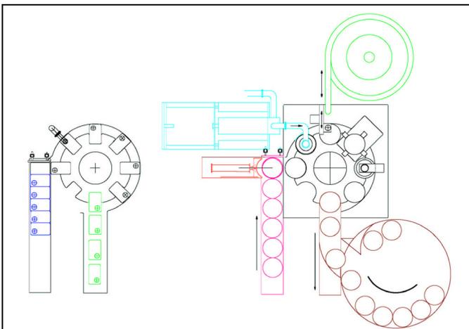
The Drawing on the left shows a typical system for the filling of 5 litre circular and rectangular section containers featuring Interchangeable Carousels, In-Feed and Out-Feed Conveyors and Cap and Lid Placing and Closing Equipment.
