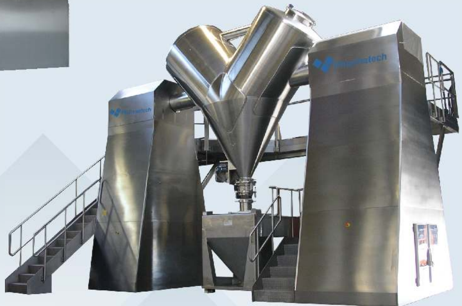
7000L V-Blender - complete with operator access gantry
