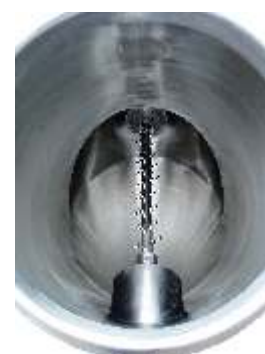
Internal view of a V Shell showing the agitator bar
