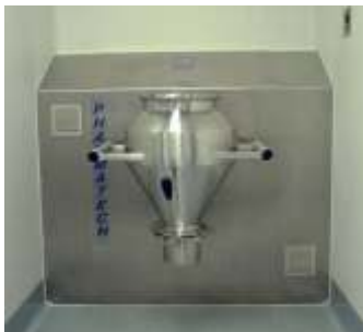
LC400 with a 100 litre double cone - blender has been modified for installation in an alcove
