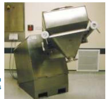
Mobile MB400 fitted with pallet truck channels
