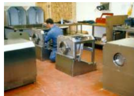
Another batch of Multiblend MB400s undergoing construction at the Pharmatech factory in Coleshill
