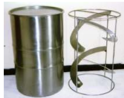
200 litre drum with removable baffles
