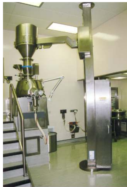
Drum Hoist with manual clamping and powered inversion. Loading a mixer granulator with a drum hoist
