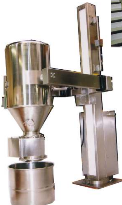
Powered Horizontal Clamping and Parallel Inversion
