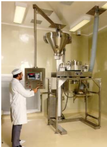
Mill Hoist with weighing system.
