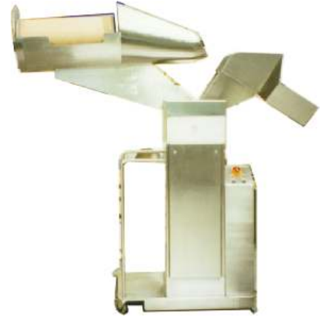
Mobile Tipper with cone chute & a chute extension
