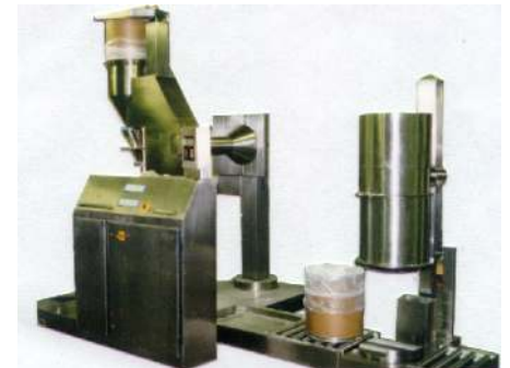
Discharge and weighing station
