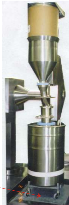
Fibre Keg discharging through the mill into a stainless steel drum
