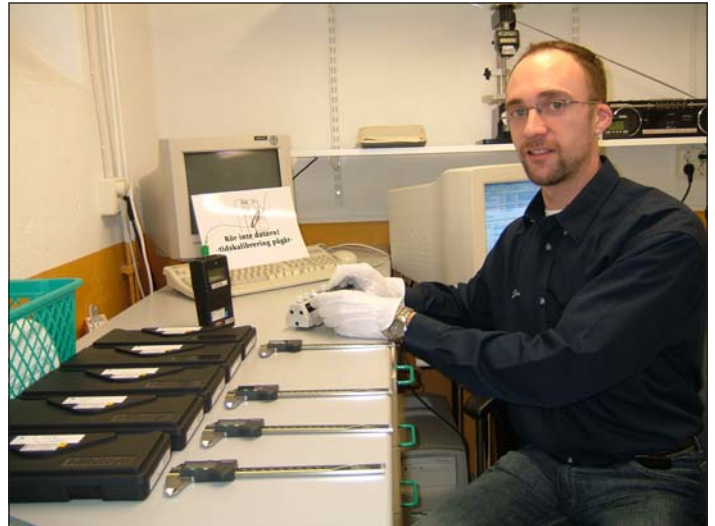
Jonas, our Calibration Manager, is calibrating callipers with the help of a gauge block ladder.
