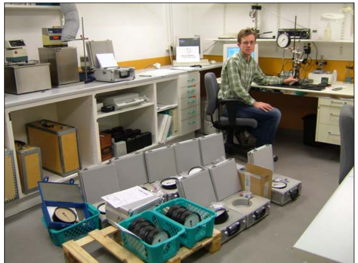
Niklas has received a major number of manometers to be calibrated. Car repair shops that control AC pressure use these manometers.
