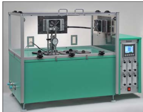
Sealed container for testing of Stress Relaxation in liquids
