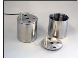
Sealed container for testing of Stress Relaxation in liquids
