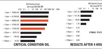
Results shown are subject to variations according to system size, flow rate, and original oil condition
