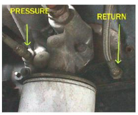
Replace with 3/8"-#4 JIC fitting. **The engine side of Fitting must be coated with thread sealant or Teflon tape.** This is the oil return, and will connect to the **OUT** port on the filter.
