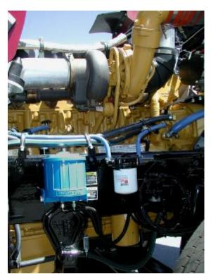
Install the filter vessel to the bracket and ensure that the mount is solid.
