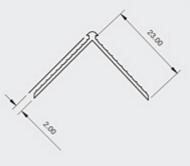
Locally manufactured from recycled plastic, Renderplas 2mm PVCu corner beads / angle beads are designed for function and speed on external and internal rendering and plastering applications. This lightweight profile is suitable on external wall insulation with a thin application of acrylic render, on plasterboard with skim plaster or for drylining / drywall systems
