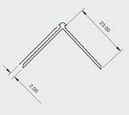
Locally manufactured from recycled plastic, Renderplas 2mm PVCu arch corner beads / angle beads are designed for external and internal arches to provide protection from impact and speed up application for a smooth regular curve on the outer edge
