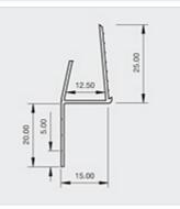
Locally manufactured from recycled plastic, Renderplas PVCu architrave shadow gap beads are designed for plasterboard to quickly and accurately form a shadow gap and provide a superior clean finish. Used at the edges of the plasterboard next to door frames, ceilings and skirting boards where the adjacent finish is designed to be seen
