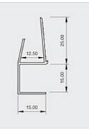
Locally manufactured from recycled plastic, Renderplas PVCu architrave shadow gap beads are designed for plasterboard to quickly and accurately form a shadow gap and provide a superior clean finish. Used at the edges of the plasterboard next to door frames, ceilings and skirting boards where the adjacent finish is hidden
