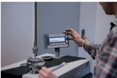
▲ Helium leakage test
